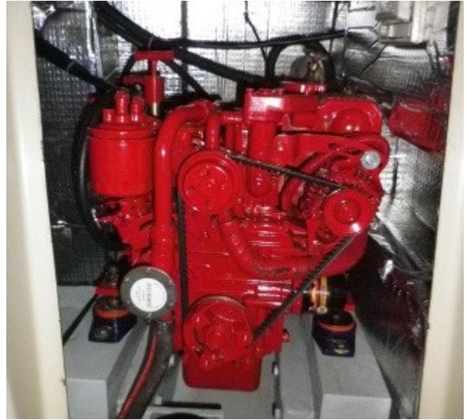
The Atomic 4 gasoline engine may be replaced by one of a range of Beta Marine diesels, from 14 to 35h.p. Since the Atomic 4 was installed as original power in everything from 25ft to 40+ ft boats, it is important to choose the correct Beta model for your boat – one size does not fit all!
