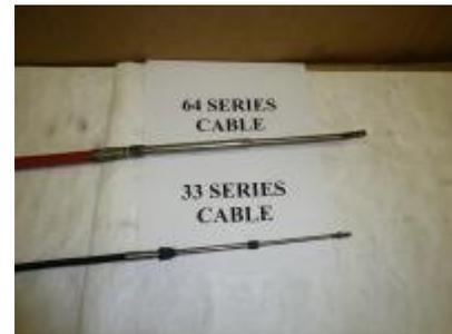
The Atomic 4 gear shift control required a heavy 64 series control cable, because of the long throw, high effort lever on the transmission. All marine transmissions now use a 33 series cable which is much smaller than the 64 series cable, with a shorter throw and mounting configuration.
